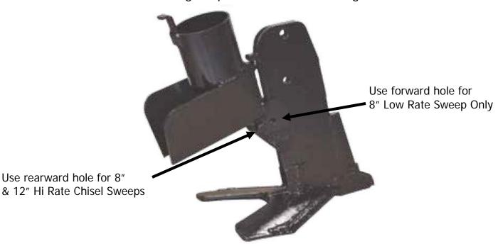
To prevent hose damage, do not torque the stover lock nut on the wing drop tube. Snug the stover lock nut so the unit can pivot when the bottom sweep bolt shears.
